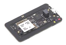
The VTAP50 from Dot Origin can selectively read and decrypt NFC pass data from iPhone or Android devices, and transfer this data to a connected system. It can also read unique IDs and secure encoded data from many RFID and NFC cards and tags, including MIFARE Classic and DESFire.
