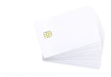
The SLE5542 is a standard, low-cost memory smartcard. It has 256 bytes EEPROM memory plus 32 x 1 bit protection memory. The SLE5542 is a fully-compatible, upgraded version of the SLE4442. Infineon has migrated the data carrier family to the IMEM CMOS technology. IMEM is conceived for security applications and offers unsurpassed physical and electrical protection schemes.
