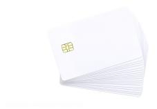
The SLE5528 is a standard, low-cost EEPROM memory smartcard with 1K bytes of available storage, with an irreversible write protection feature and a 2-byte programmable security code. The SLE5528 is a fully-compatible, upgraded version of the SLE4428.
