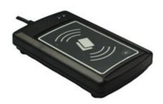
The ACR1281U-C2 from ACS is a 13.56MHz contactless reader device that appears to the host device/PC as a keyboard, and automatically reads the chip serial number (CSN) of each card when presented.
