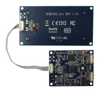
The ACM1252U-Y3 contactless and NFC reader module from ACS is a 13.56 MHz USB NFC solution that supports a wide range of technologies including NFC (card reader/writer, card emulation, and peer-to-peer communication), ISO 14443, ISO 18092, FeliCa and various NFC devices.
